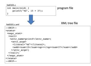
Fig. 5. Example of input and output of the parser
